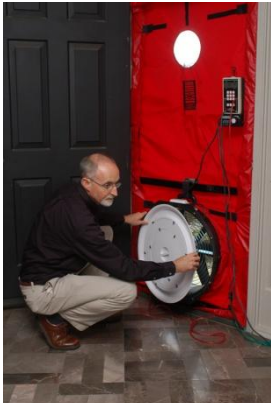
Blower Door to determine total air leakage
