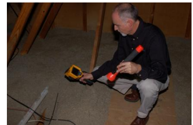
Auditor with infrared camera to find specific location of air leaks.
